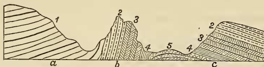
FIG. 1.—Section from Stone mountain at Little Stone gap to Powell mountain. a , Slope of Black mountain; b , Stone mountain; c , Powell mountain; 1, Coal Measures; 2, Quinimont group; 3, Lower Carboniferous; 4, Devonian; 5, Upper Silurian; 6, Lower Silurian.
